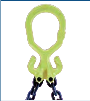
Fig. 1. The GrabiQ Master Grab combines a master link, master link connectors for two legs of chain, and two shortening hooks into a single fitting. The shortening hook can also be used to create loop legs.
